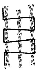
FACE AND BACK WARP YARNS WEAVING ONE END AS ONE MIDDLE WARP YARNS WEAVING TWO ENDS AS ONE BINDER WARP YARNS WEAVING TWO ENDS AS ONE
